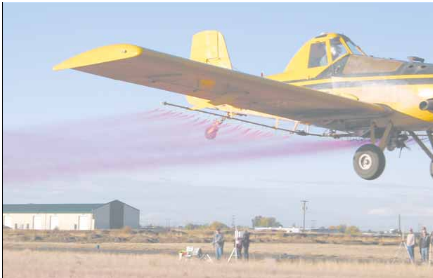
An aerial applicator releases water-soluble fluorescent dye over an absorbent string at the Moses Lake Municipal Airport. The string is analyzed to determine the spray patterns. The information helps pilots adjust pressures and nozzles to assure that they are applying crop protection and nutrient materials where they are needed and to avoid drift. The tests are part of a national program called Operation SAFE, which stands for Self-Regulation Application and Flight Efficiency. (Photo courtesy of Matthew Weaver, Columbia Basin Herald)
